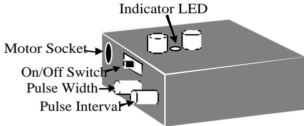
**On/off:** Push slide switch to left to turn on (indicator LED will light), right to turn off (indicator LED will extinguish).
